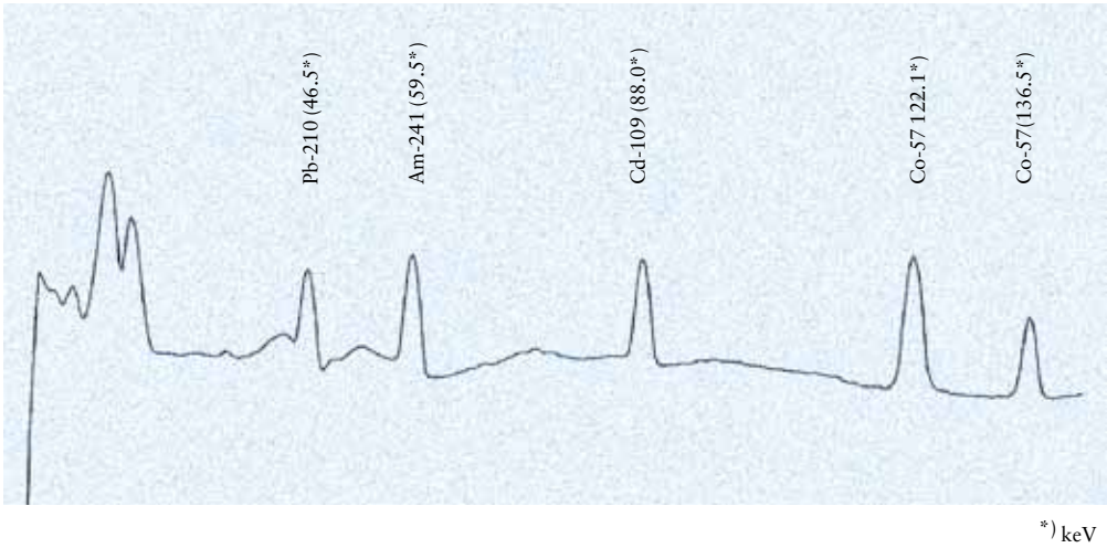
A typical gamma spectrum for the NG4 radionuclide mixture
