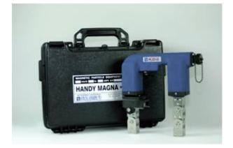
**MP-A2L** products use testing method by utilizing the Yoke Method, to magnetize with some or all of test flaws placed between
